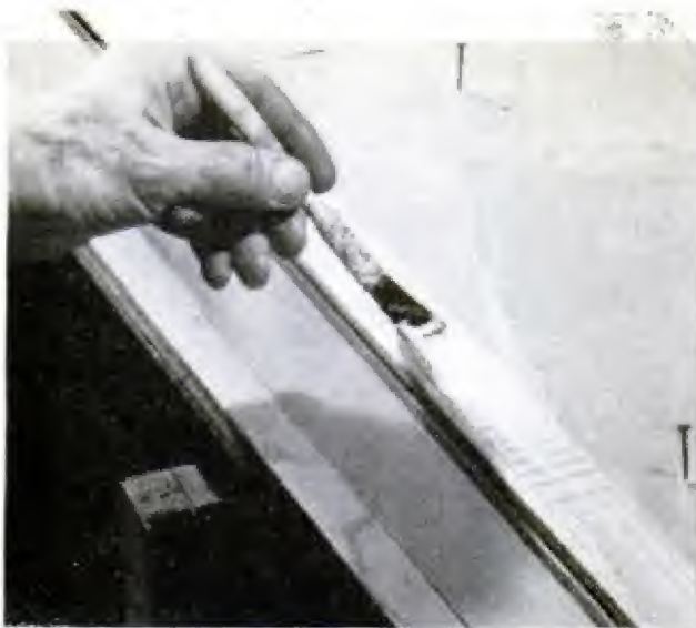
WATER-SOLUBLE GLUE , mixed with fine sawdust, is brushed into the kerfs, serves as an effective filler
